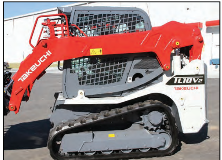
Vertical Lift Path for Balance and Stability
